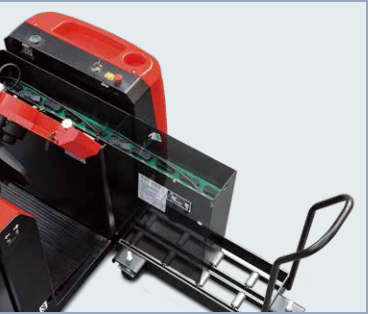
Side battery changes is standard feature
