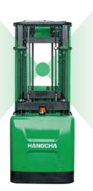
The mast with its upper surface low from the ground offers a wide view and good driving vision.
